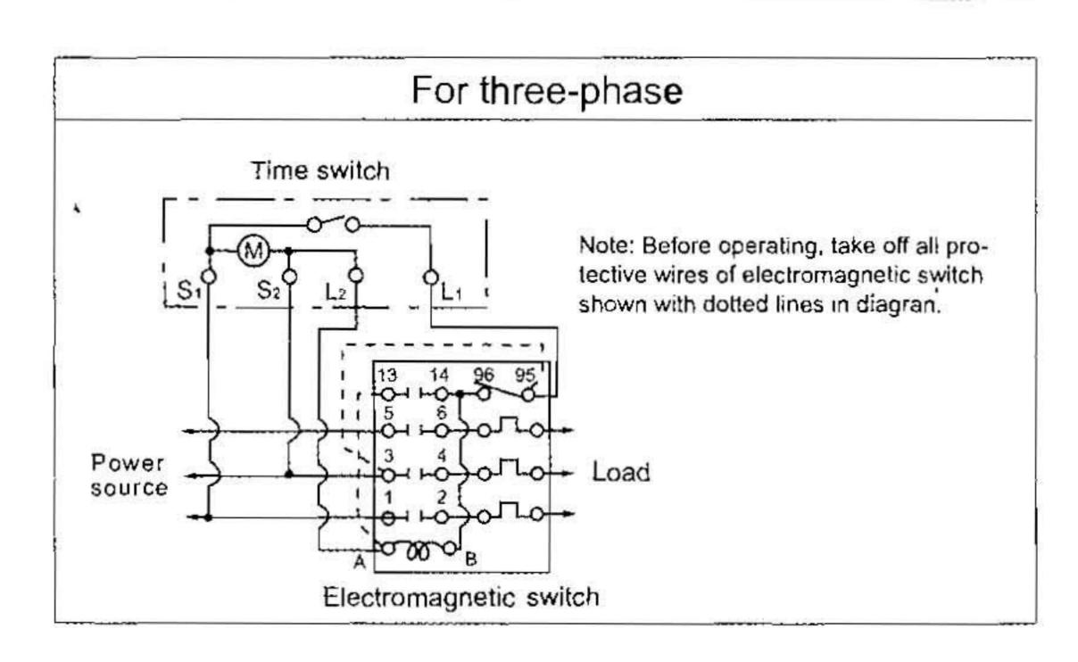
verien a nearer is used as a load, be sure to insert a merinoswitch into the load circuit.
